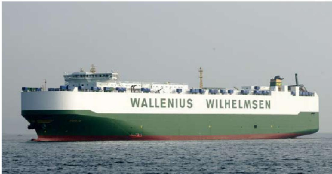
The LCTC (Large Car Truck Carrier) m/v FIDELIO has a capacity of 8,000 cars or a combination of 3,484 cars and 468 buses. With her 227.8 metres this capacity makes her one of the largest car carriers in the world. The vessel is built to the highest class of Lloyd's Regis-
